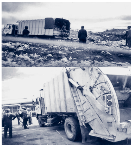
FIGURE. Box-type (top) and hydraulic compactor (bottom) refuse-collection trucks — Bulawayo, Zimbabwe, 2003
