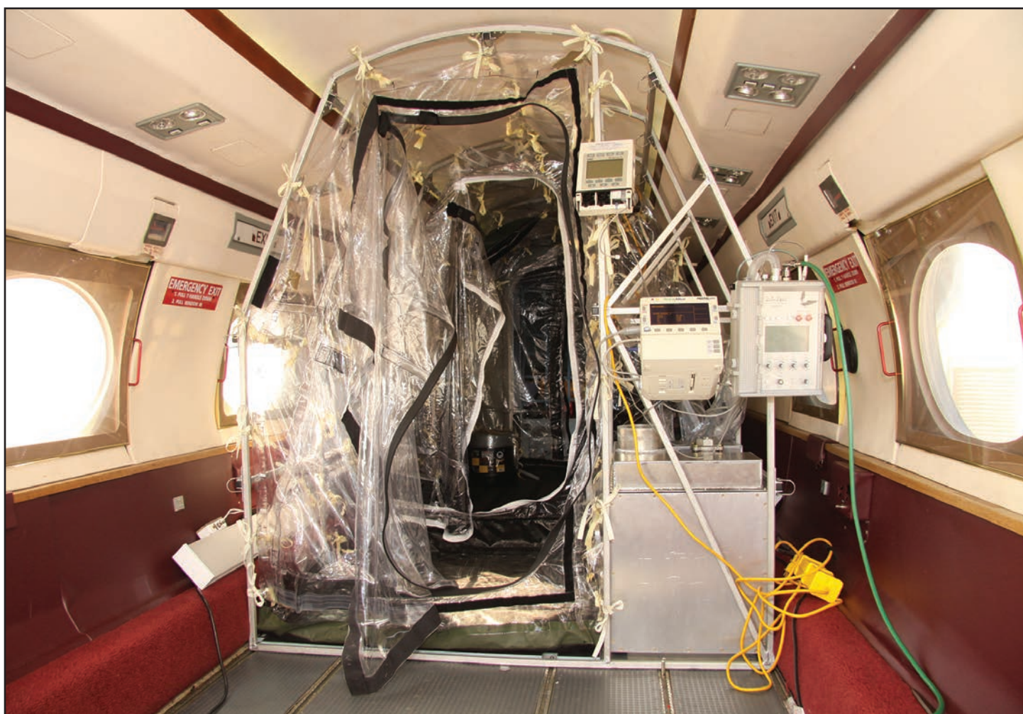
FIGURE 2. The Aeromedical Biologic Containment System installed in a Gulfstream III aircraft*
