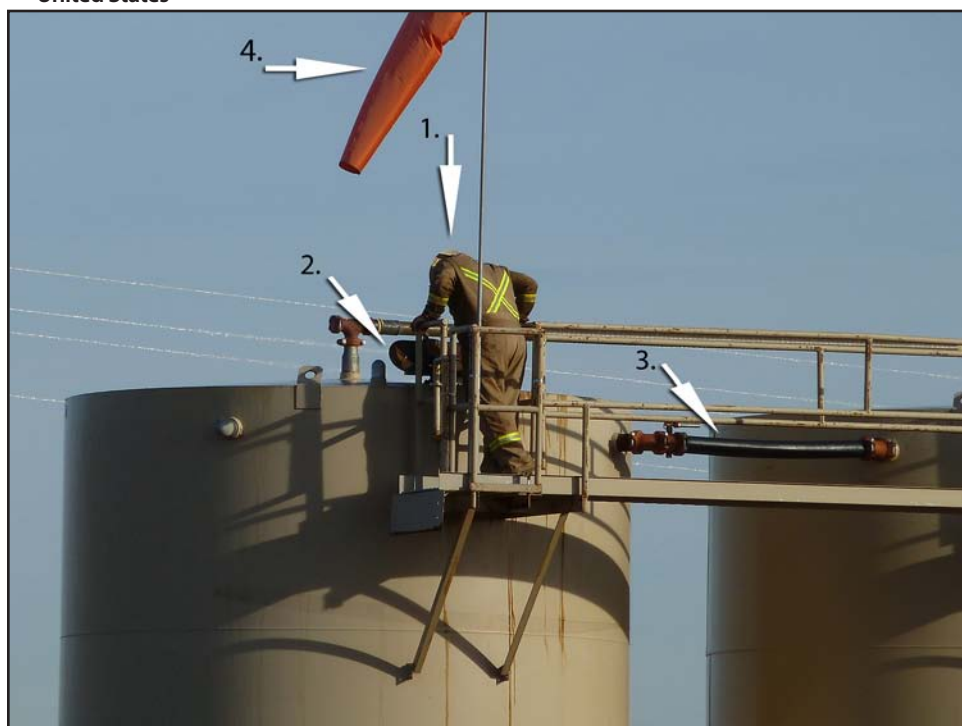
FIGURE. An oil field worker manually gauges the level of process fluid in a fixed production oil tank* — United States
