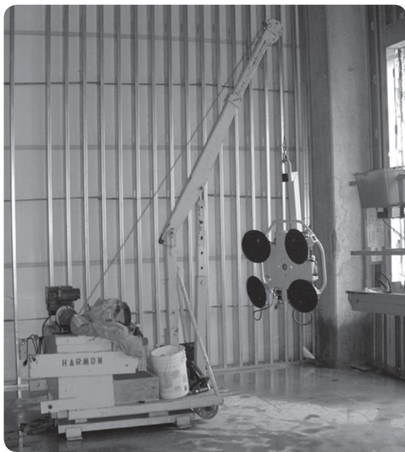
Power vacuum lifter avoids manual lifting
