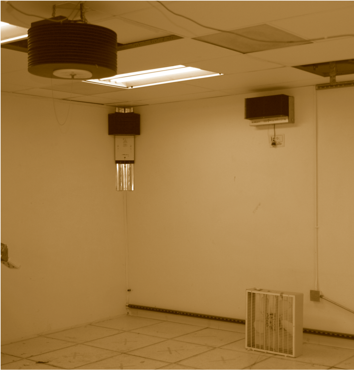
Figure 2. Simulated healthcare UVGI room, University of Colorado. (Courtesy of Professor Shelly L. Miller, University of Colorado, Boulder, Colorado).
