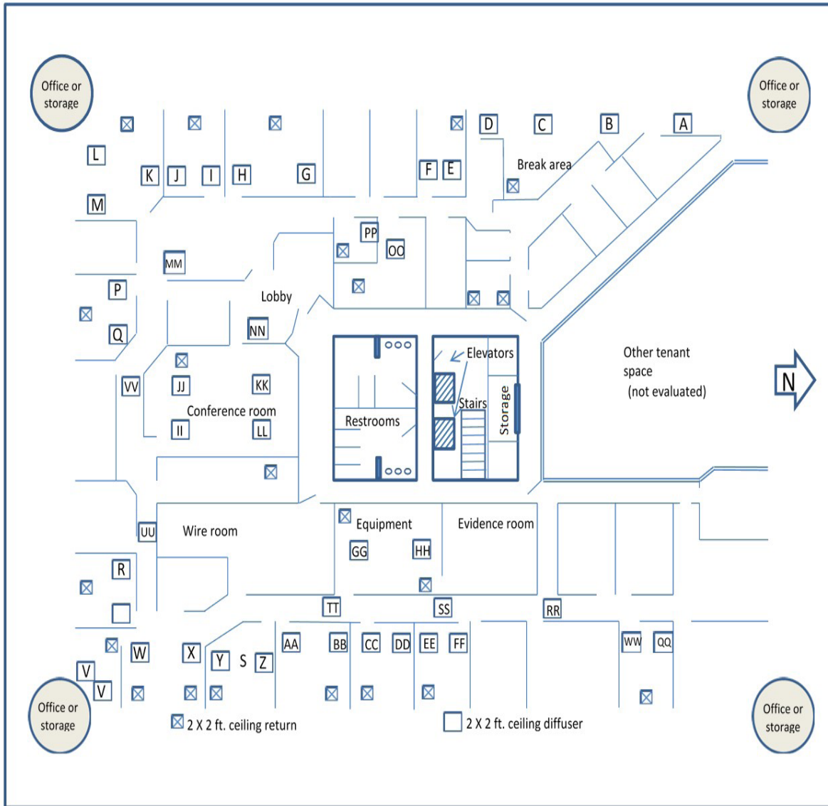
Figure B1. Office diffuser locations, seventh floor
