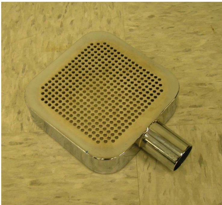
Figure 9: Rectangular side exhaust hood
