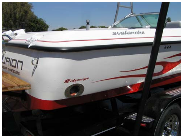
Figure 3 2005 Centurion Avalanche Ski Boat with Sideswipe Exhaust
