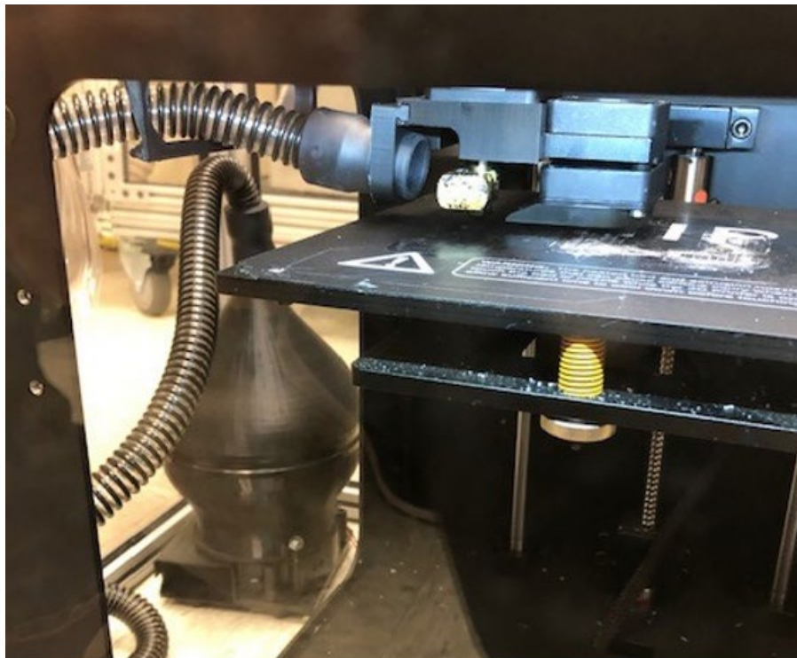
Figure 2: 3D Printer A with LEV control attached. Photo by NIOSH.
