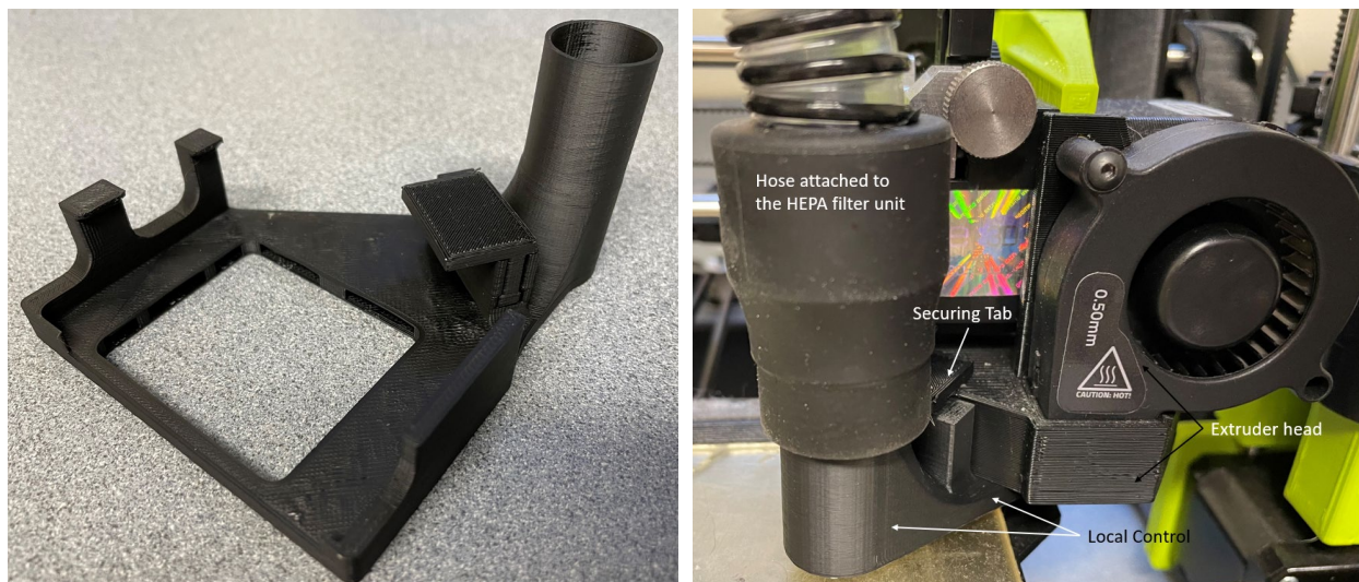
Figure 5: 3D Printer B LEV control with tab inserted (left) and control attached to the 3D printer extruder head (right). Photos by NIOSH.
