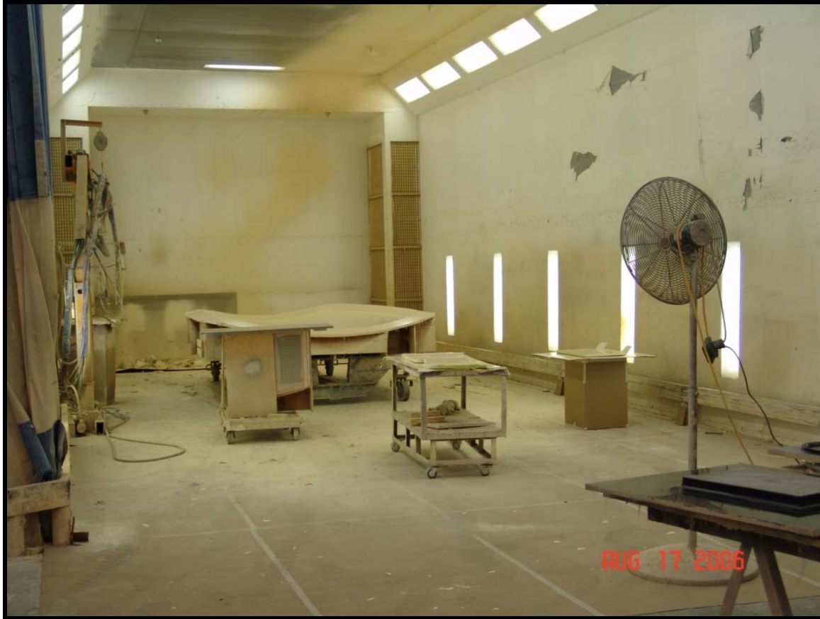
Figure 2: Gelcoat booth containing small part molds during the curing process
