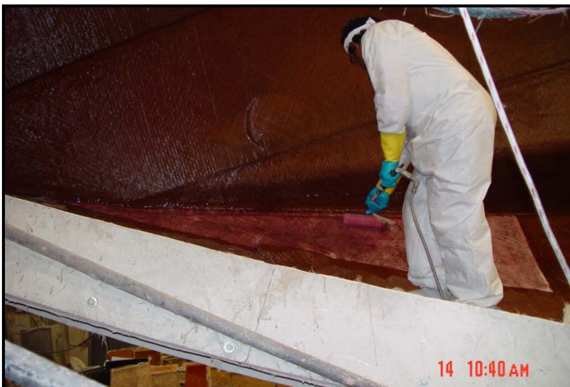
Figure 3: Large part laminator releasing resin using the pressure-fed perforated rollers
