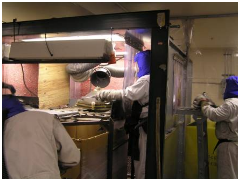
Figure VII – Electron Gun Removal in Glass Breaking Operation
