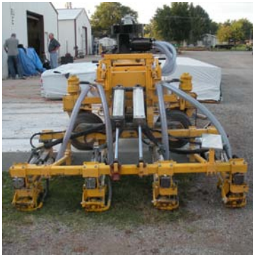
Figure 1 - E-Z Drill model 210-3 SRA four-drill, self-propelled, on-slab dowel-pin drill
