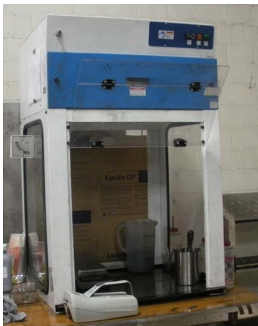
Figure 7. The ventilated enclosure used for product transfer.
